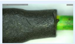
Terminal insulation cracks identified during inspection at 65x magnification
